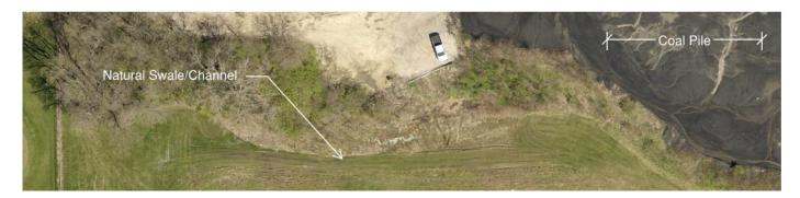
The capacity of this channel was assessed to determine its ability to convey stormwater without eroding. The existing channel dimensions (area, wetted perimeter) were taken from survey data provided by Beals-Moore and Associates, Inc. (2016) and used to determine capacity and shear stress at the 1000-year storm depth:
